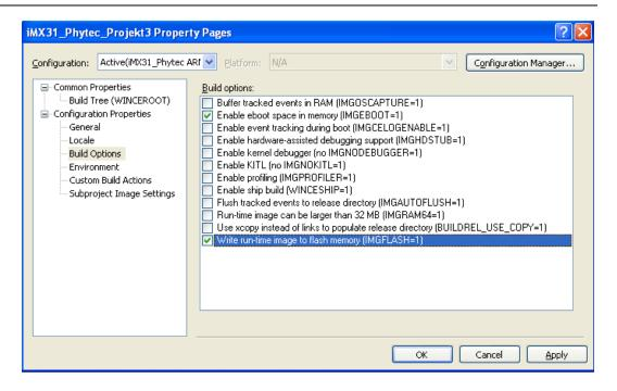
In the Properties dialog select *Configuration Properties* and *Build Options*. Check the "Write run-time image to flash memory" and rebuild the solution.
